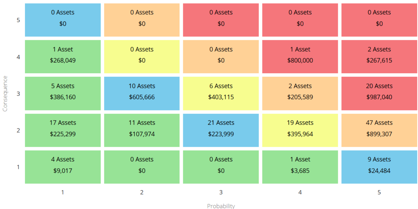
Figure 93 Risk Matrix: Misc. Machinery & Small Equipment
