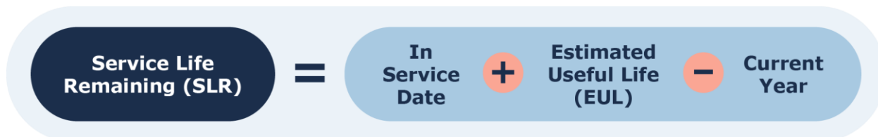
Figure 7 Service Life Remaining Calculation
