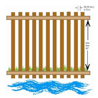
Figure 6: Vertical and horizontal member spacing
